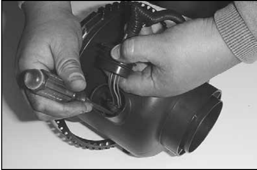
10. Slide the rubber grommet back and disconnect the primary mass air sensor electrical connection, using a flat blade screwdriver.
