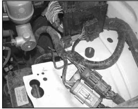
15a. On vehicles without cruise control, install the rubber mounted stud onto the vehicle as shown.
