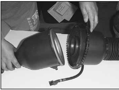
9. Open the air cleaner assembly and isolate the mass air sensor assembly.
