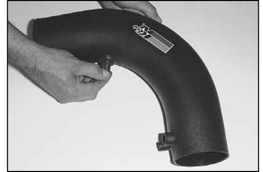
20. Using the provided grommet, install the air temperature sensor into the K&N® intake tube.
