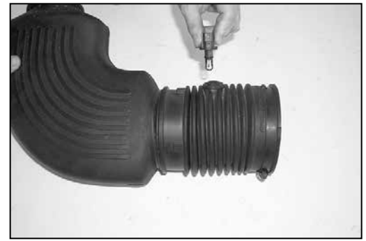
19. Remove the air temp. sensor from the stock air intake tube as shown.
