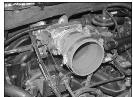
23. Using the provided hose clamp, attach the silicone hose (08724) to the throttle body.
