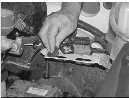
13. Remove the two air box mounting grommets from vehicle as shown.
