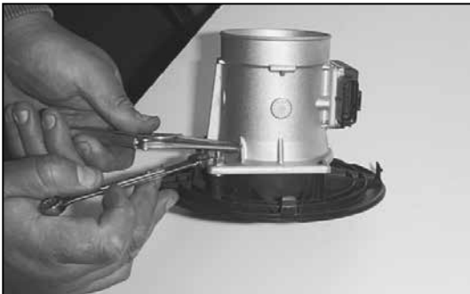
12. Using a pair of small vise grips or pliers, hold the stud while using a 10mm wrench to loosen the nuts, then remove the mass air sensor from the retaining plate.
