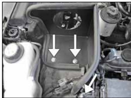
18. On vehicles equipped with cruise control, set the heat shield into position on the air filter mounting bracket. Then secure the heat shield with the provided hardware as shown. NOTE: Be sure the mounting bracket and cruise control are secured together.
