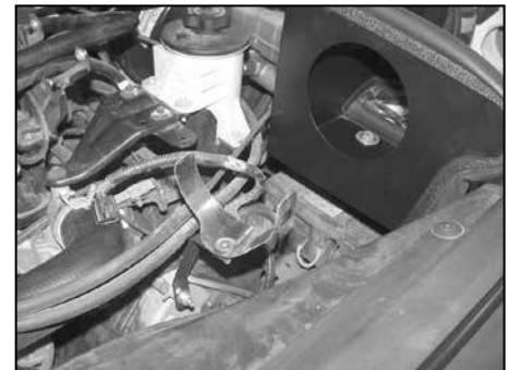
22. Install the saddle bracket assembly onto the protruding stud as shown, secure into place using the provided hardware.
